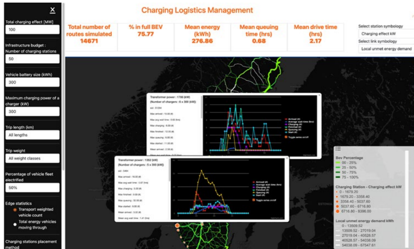
Tool that allows the map-based exploration of the results of EV routing and charging simulations. The timeseries show the variability of charging queue and charger utilization in space and time through two charging stations as examples.
